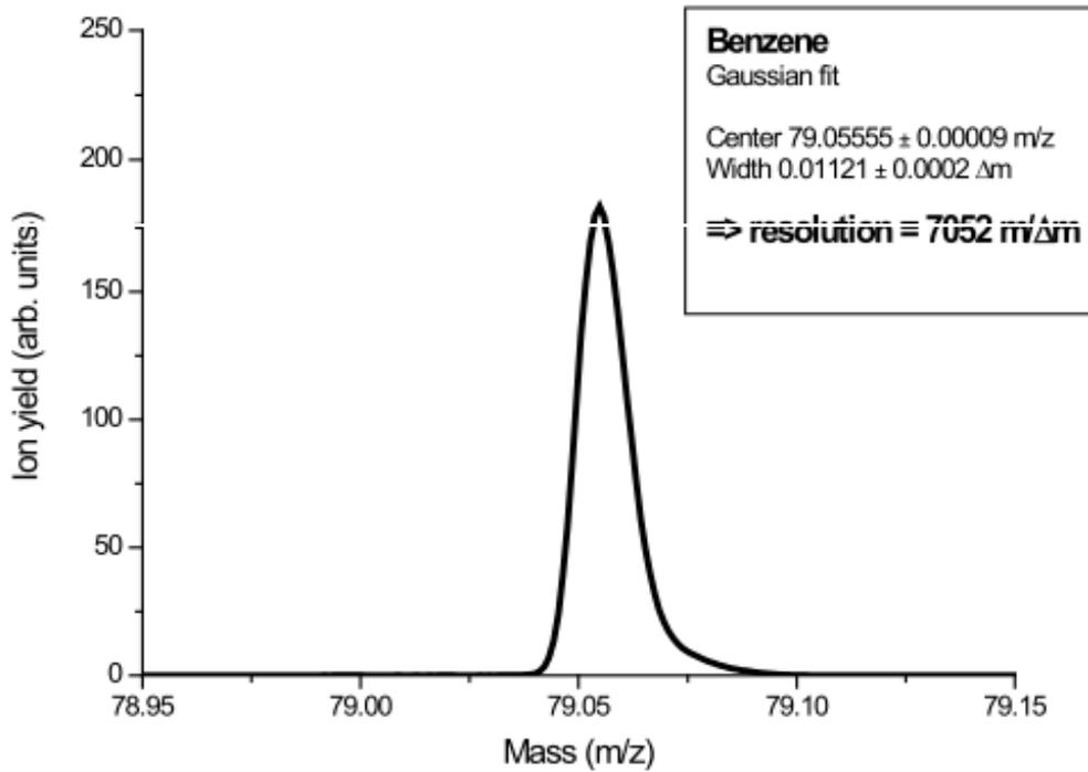
In the above example, a peak is shown for benzene. The information box quotes a mass resolution value of 7,052 using a 'Gaussian fit' (curve not shown). However, if one measures the full width at half maximum of the actual peak (and not a mathematically generated curve), it measures somewhere between 5,600 and 5,750 and is not 7,052.
