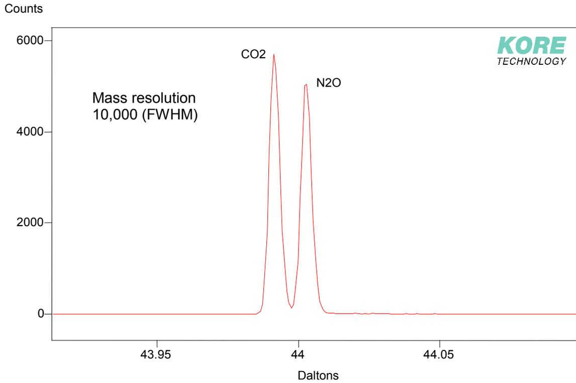
Data obtained from the new TOF spectrometer, showing baseline separation of CO<sub>2</sub> and N<sub>2</sub>O at mass 44. Mass resolution 10,000 (FWHM). This data was taken using an electron impact ion source and an instrument with an aperture at a focal point in the ion optics. This reduces the transmission but increases the mass resolution.
