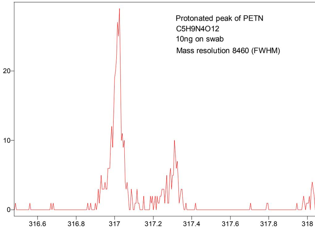
**Example of high mass resolution at reduced transmission (aperture)**
